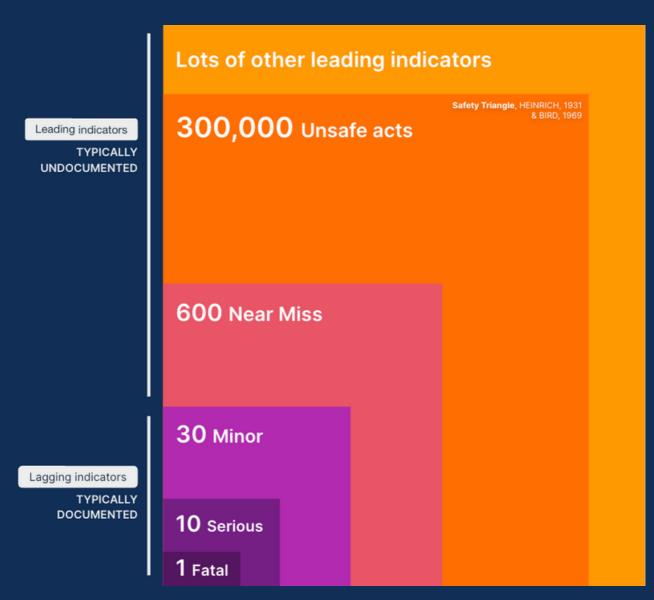
Designed based on the accident triangle, also known as Heinrich's triangle or Brid's triangle.
